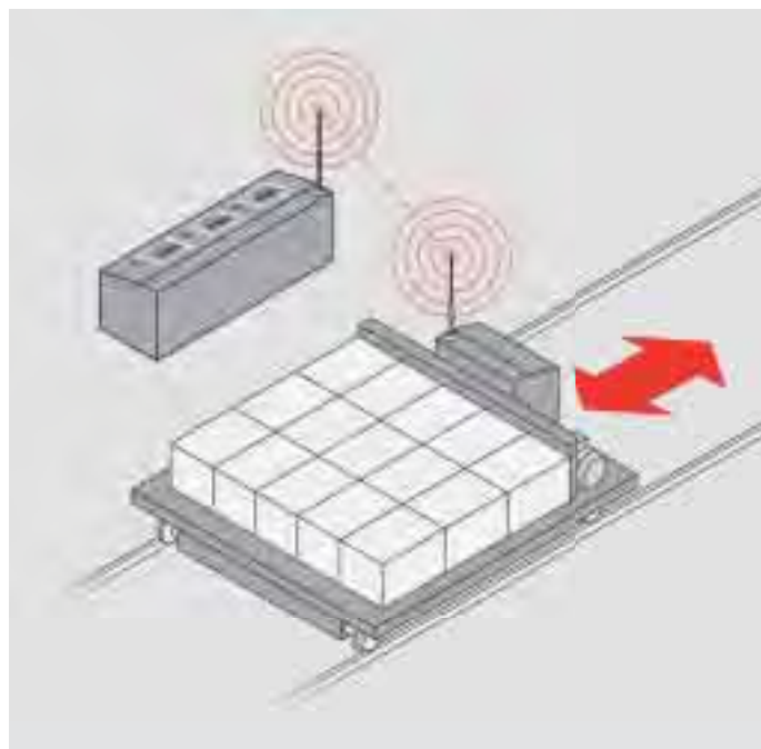
Wireless signal transfer via InduraNET p in plants with moving parts.
